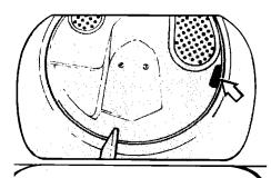
A sensor on the back the drver drum "feels" the amount of moisture in the load. When the dryness you have selected is reached, the dryer automatically shuts off.
